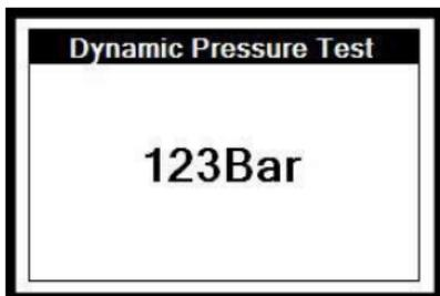
√Accelerate or decelerate the engine to check if the pressure varies correctly.
